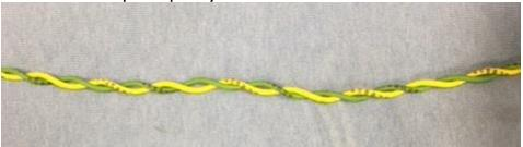
Notice the gaps between the wires and also how the twist length is not consistent. Gaps in poorly twisted wire will result in large impedance fluctuation. In addition, poorly twisted wire will have much higher return loss. High return loss means less signal being received and higher data error rates. Using poorly twisted cables is similar to speaking with someone on a cell phone when you have only 1 bar of signal. Much of the message is missing or garbled.
