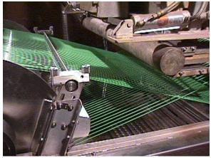
Wire in a typical "figure-8" pattern under an irradiation beam
