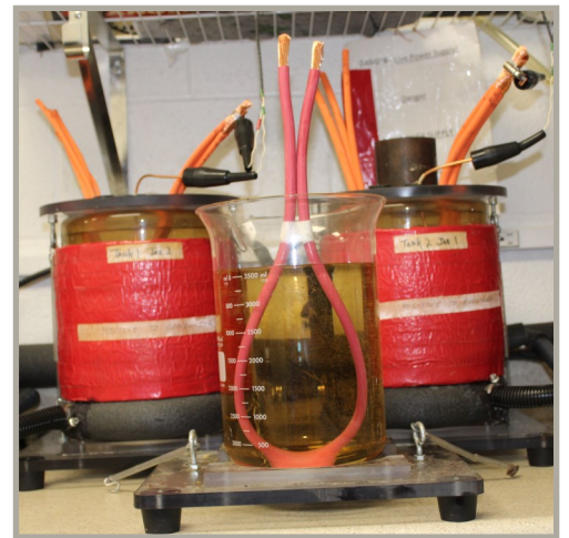
Cables Immersed in Fluid per 19642
