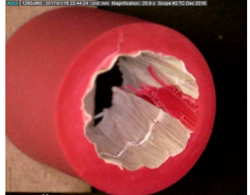
EPDM sample with incomplete tape wrapping of the conductor
