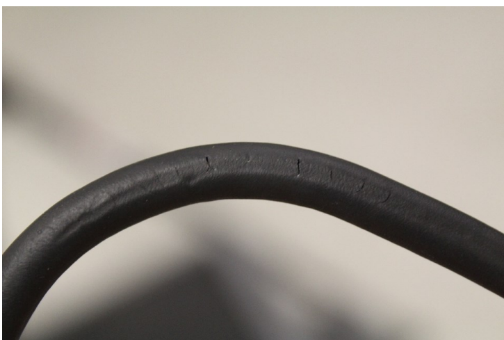
EPDM samples cracked in many places after 150C heat age
