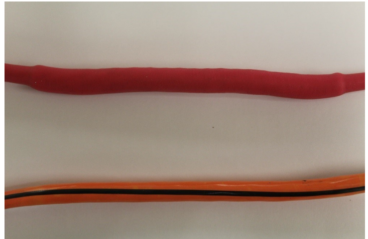
Top: EPDM sample. Bottom: EXTRAD sample
